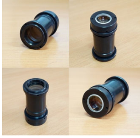
Fig. 2 Optical system of star tracker experimental model
