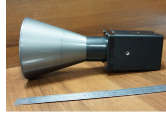
Fig. 4 Experimental model of star tracker with the hood
